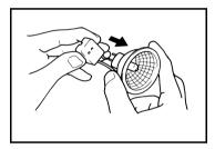
Insert a new Projection Lamp so that the mark on its base is facing upwards. Make sure that the new Projection Lamp is inserted securely so that there is no gap between the projection Lamp and the Lamp Socket.
